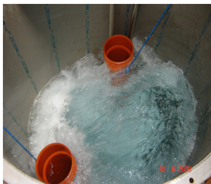
Test of venting the space under the weir using 2x225mm pipes
