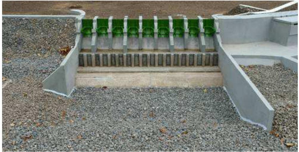
Scale model (1:80) of the spillway for the Tocoma Hydroelectric Project, Venezuela, with downstream wing walls and concrete protection of the upstream slope of the pre-excavated plunge pool
